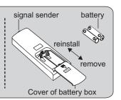
3. Reinstall the cover of battery box.
