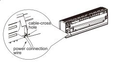
Remove the wire clip; connect the power connection wire to the wiring terminal according to the color; tighten the screw and then fix the power connection wire with wire clip.
