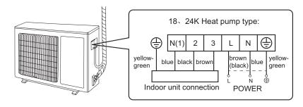
2. Fix the power connection wire and signal control wire with wire clip (only for cooling and heating unit).
