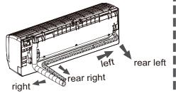
2. When select leading out the pipe from left or right, please cut off the corresponding hole on the bottom case.
